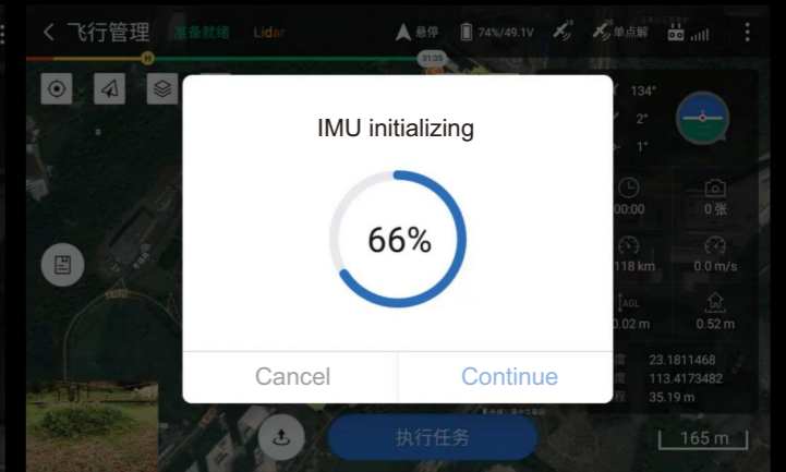
c. LiDAR self-check and IMU initializing on GCS(no need 8-shape check).
