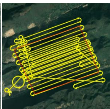
smart elevation partition for hilly terrain
